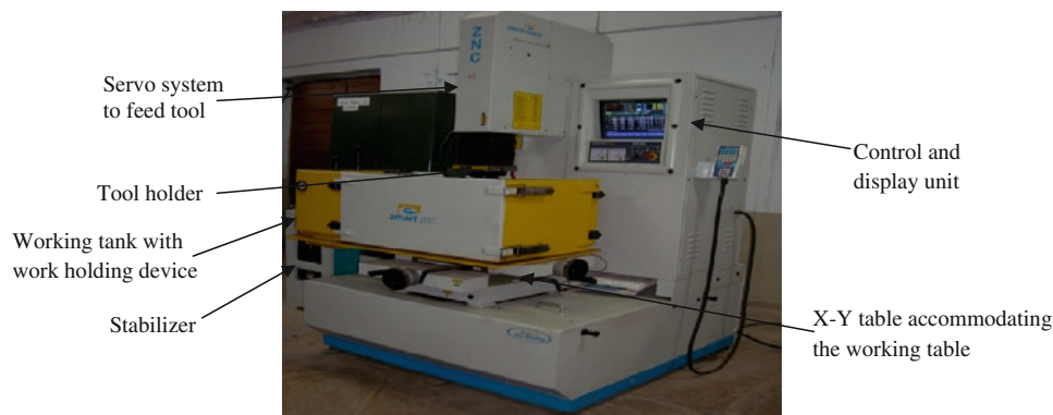
Fig. 1 Die-sinking EDM machine
